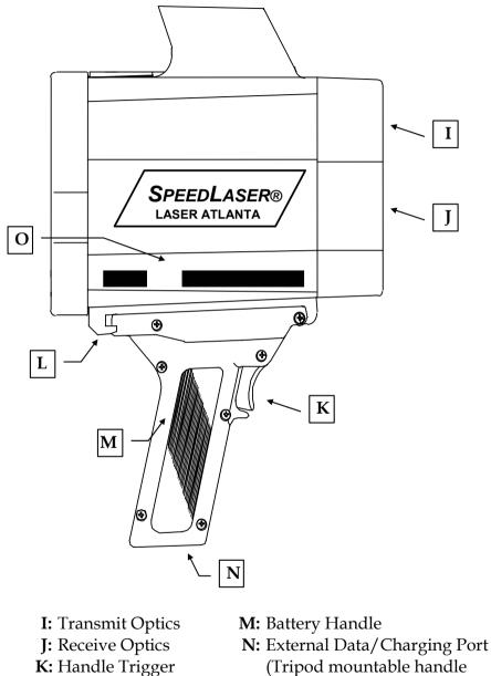
(Tripod mountable handle has data port on the side)
