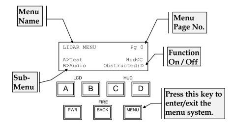
For each menu choice, on the outside left or right edge of the LCD is the letter matching the key to be pressed to activate the option. Between each key letter and its corresponding description is a symbol. The meanings of the symbols are as follows:
