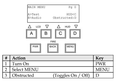
Set to ON when firing the LIDAR through the patrol vehicle window, or when RAIN, SNOW, FOG or other OBSTRUCTIONS are present.
