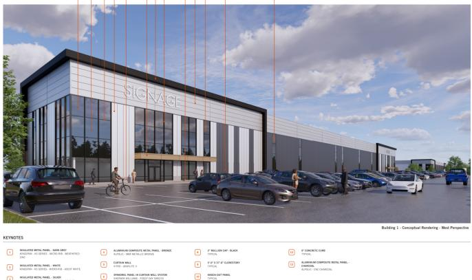
The elevations at 12668 Dixie Road have a clean modern look with accent banding along the parapets and contrasting copper-coloured canopies. The entrances are clearly visible and inviting, highlighted by Aluminum Composite Metal accents, glazing and canopies.
