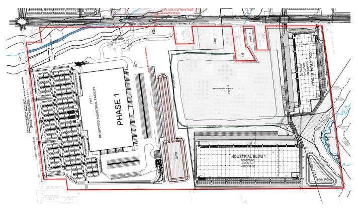
Access for passenger vehicles and trucks is consolidated at the street to minimize the number of curb cuts required; however, passenger vehicles split away from the heavy vehicle traffic upon entry to the site and remain separated so they can circulate independently within the parking areas safely.
