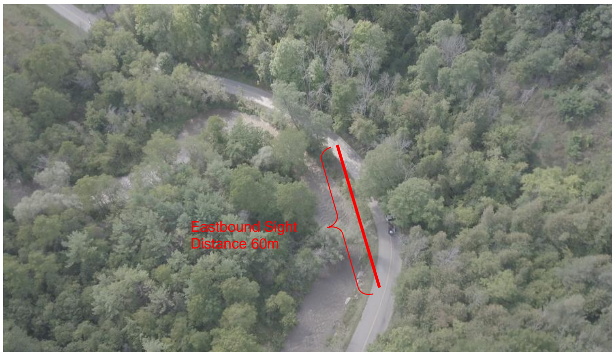
Figure 6: Sight Distance for the Curve
