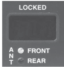
Figure 4.2c The FRONT and REAR antenna lights.
