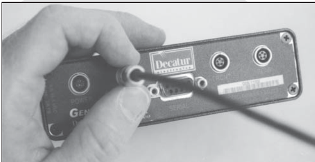
Figure 2.2b Align the red dot on the connector with the red dot on the computer receptacle.
