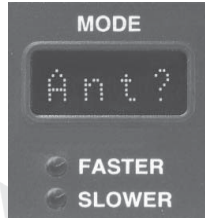
Figure 3.2a If no antenna is connected, Ant? displays.
