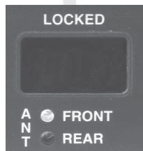
Figure 3.2b When the FRONT light illuminates, the FRONT antenna is transmitting.
