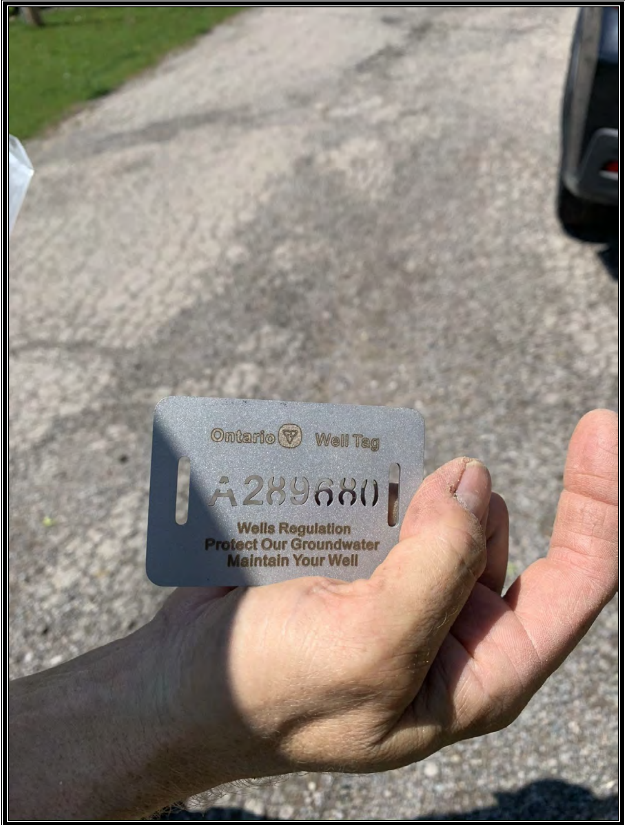
Photograph 9: MECP well tag installed with monitoring wells on-site
