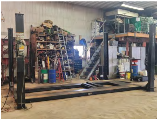
Picture 45: View of the hydraulic hoist in the Maintenance Barn.
