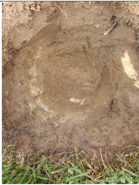
IMAGE 8 COMPLETED DISTURBED TEST PIT
