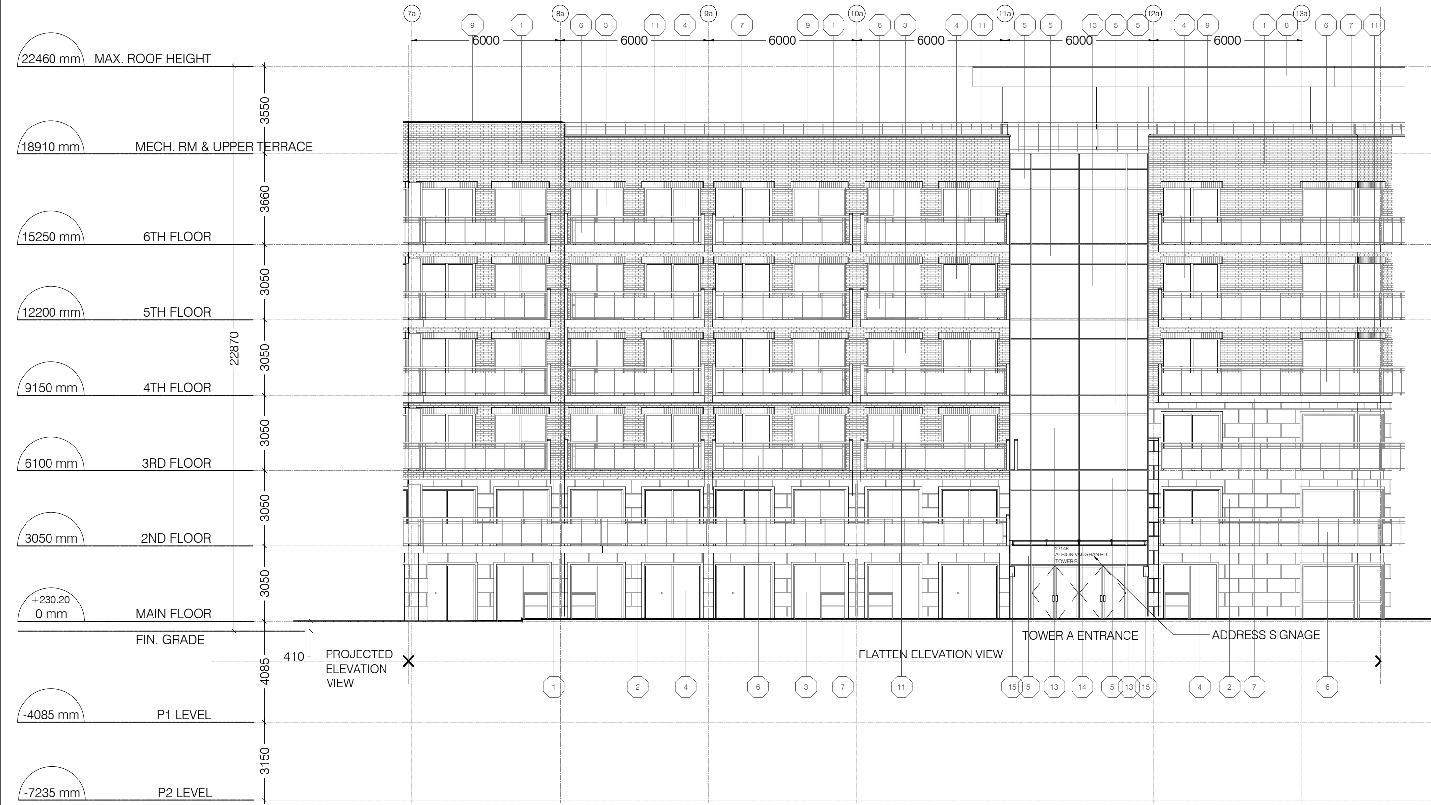
1 EAST ELEVATION - TOWER A A3.1 SCALE: 1:150
