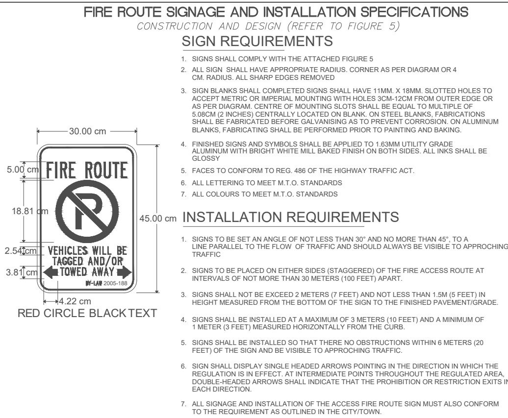
4 FIRE ROUTE SIGN DETAIL SCALE: NTS
