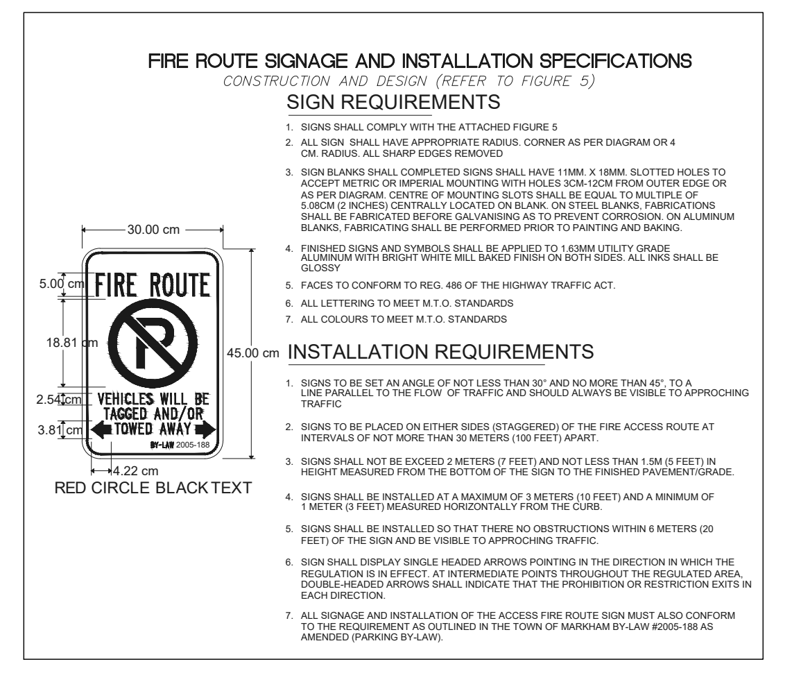
3 FIRE ROUTE SIGN DETAIL SCALE: NTS
