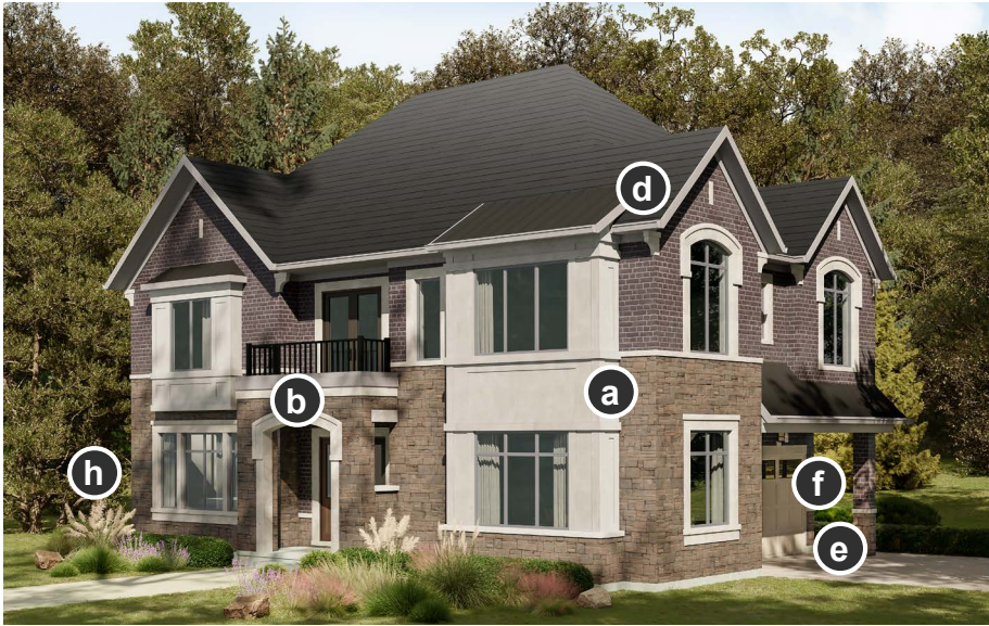
Figure 3.8d - The main entry, garage, and porch on Gateway Dwellings should be oriented to address the short (front facing) street frontage where the flankage faces a collector road
