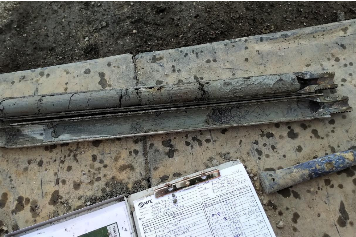
Photograph No. 2 – View of the native clayey silt till observed at borehole MW116-22, advance on the east side of the storage barn.
