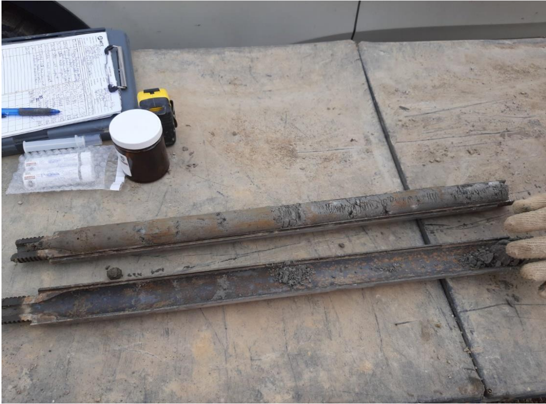
Photograph No. 9 – View of the native silt till observed at borehole MW124-22, advanced on the north side of the storage shed.
