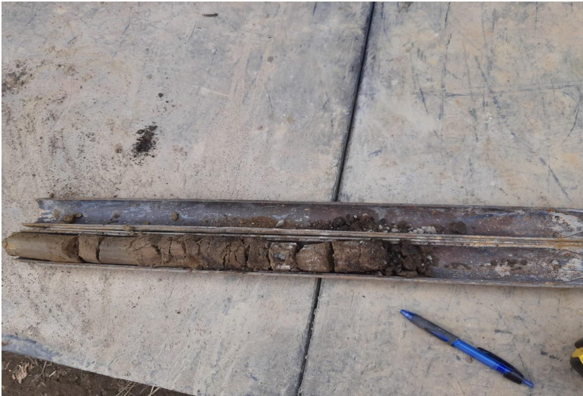
Photograph No. 8 – View of the fill material and underlying clayey silt till observed at borehole MW123-22.
