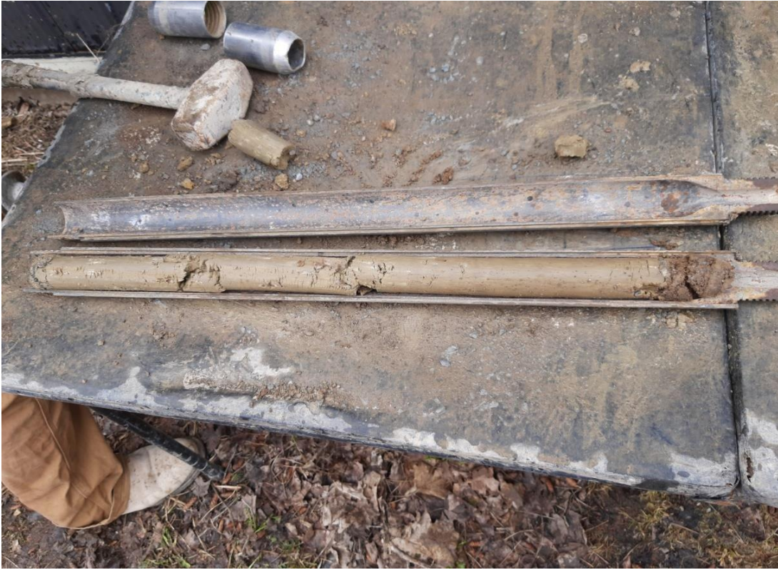
Photograph No. 5 – View of the native clayey silt till observed at borehole MW122-22, advance on the south side of the storage shed.
