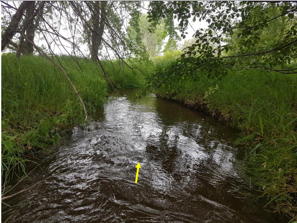
Bank angles ranged from 30° to 60° with minor undercutting observed. Average bankfull width and depth was 3.36 m and 0.65 m, respectively.
