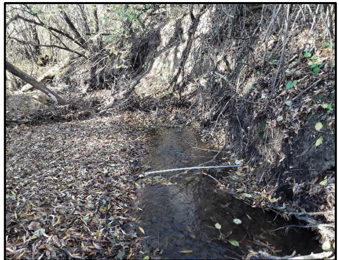
Photograph 24. Location 21. Reach WHT-2 North-South Tributary Downstream view of valley wall contact on right bank. Undercutting and till observed at the valley toe. View: US Date Taken: November 8, 2022 Site: 12522 & 12306 Torbram Rd, Caledon ON
