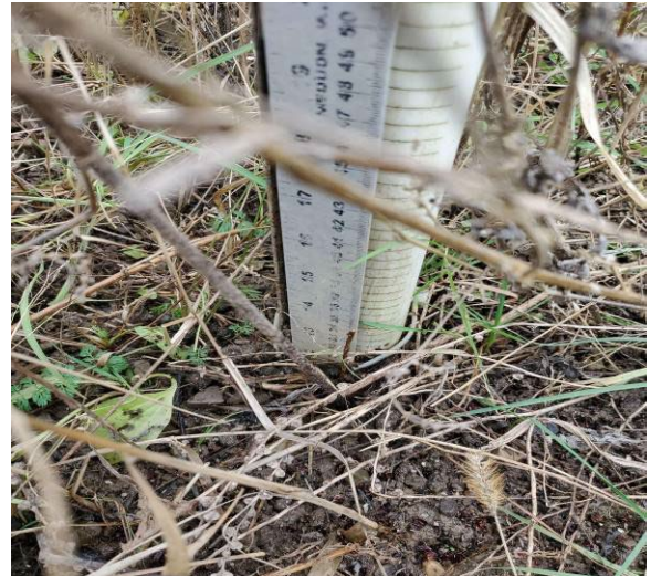
Photo 19: A closer view of the staff gauge at streamflow station SF7-17 taken on December 9, 2022. Very low water levels were observed.
