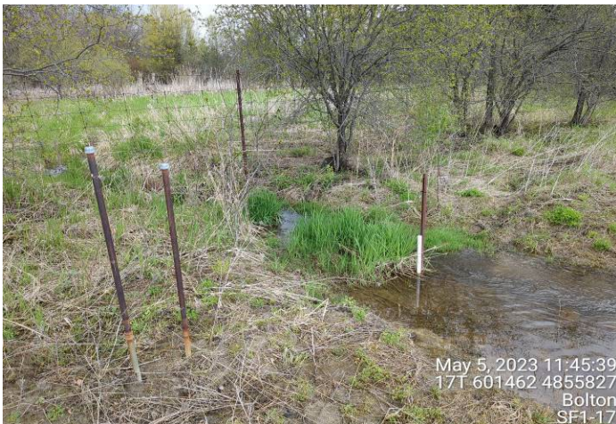
Photo 3: A view of streamflow station SF1-17 taken on May 5, 2023. Piezometers and staff gauge were observed in good condition.
