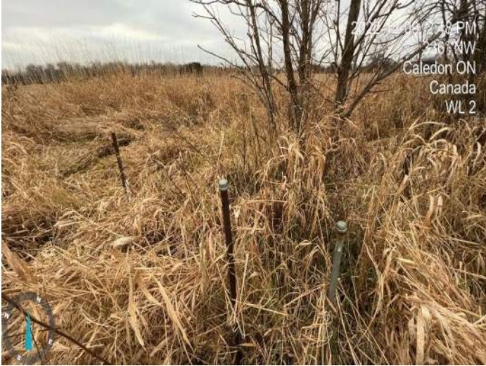
Photo 39: A view of the wetland station at WL2-17 taken on December 9, 2022. Piezometers were observed in fair condition. Staff gauge is observed behind the piezometers.
