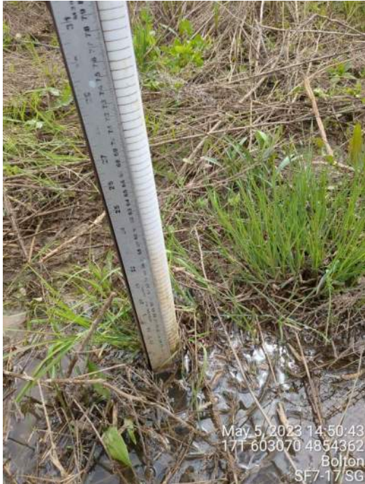
Photo 20: A closer view of the staff gauge at streamflow station SF7-17 taken on May 5, 2023. Higher water levels compared to December's visit were observed.
