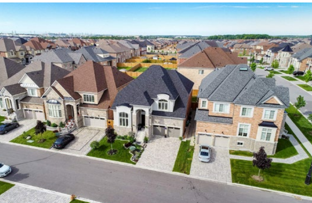
Roofscapes should vary in slopes and articulation, where possible, to contribute to the creation of interesting skyline streetscapes
