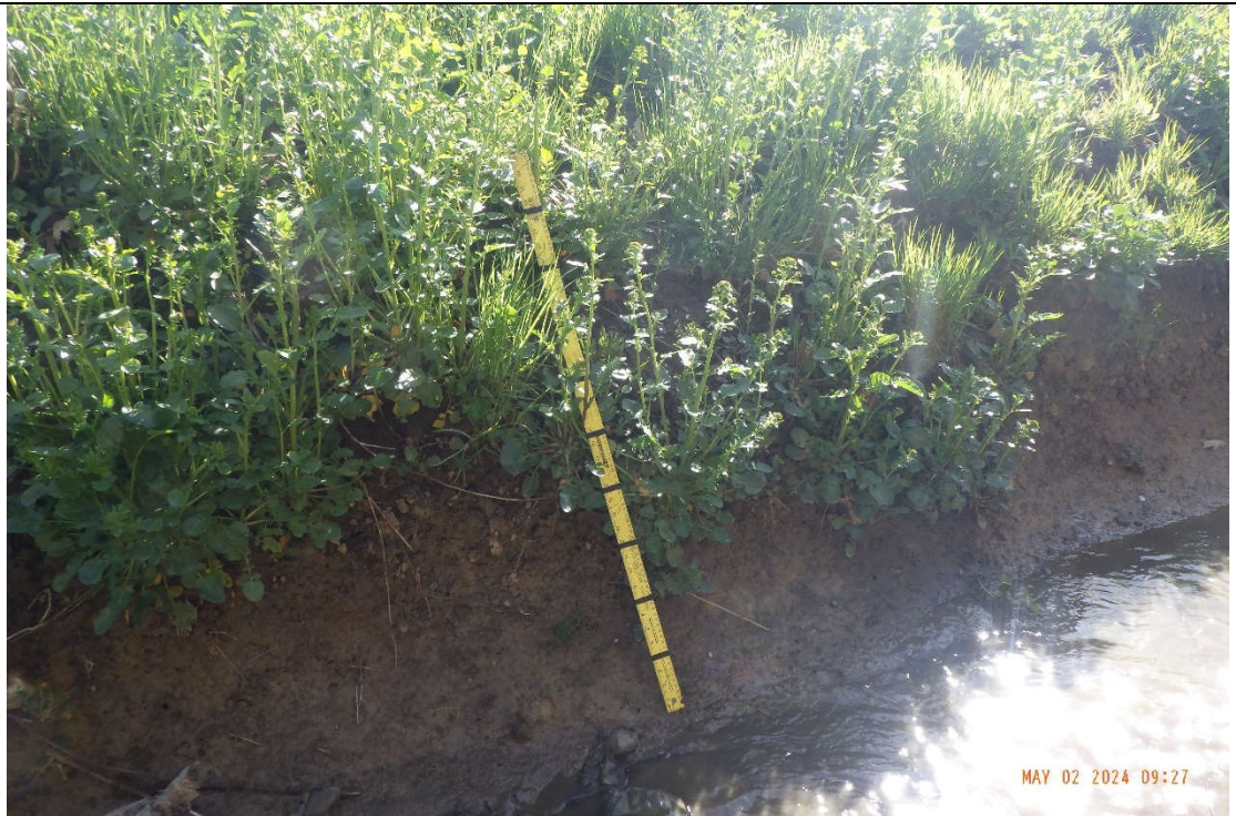
The bank substrate consisted of clay/silt and sand. Bank angles ranged from 60 – 90 degrees.
