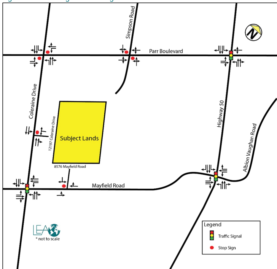
Figure 3-1: Existing Lane Configuration
