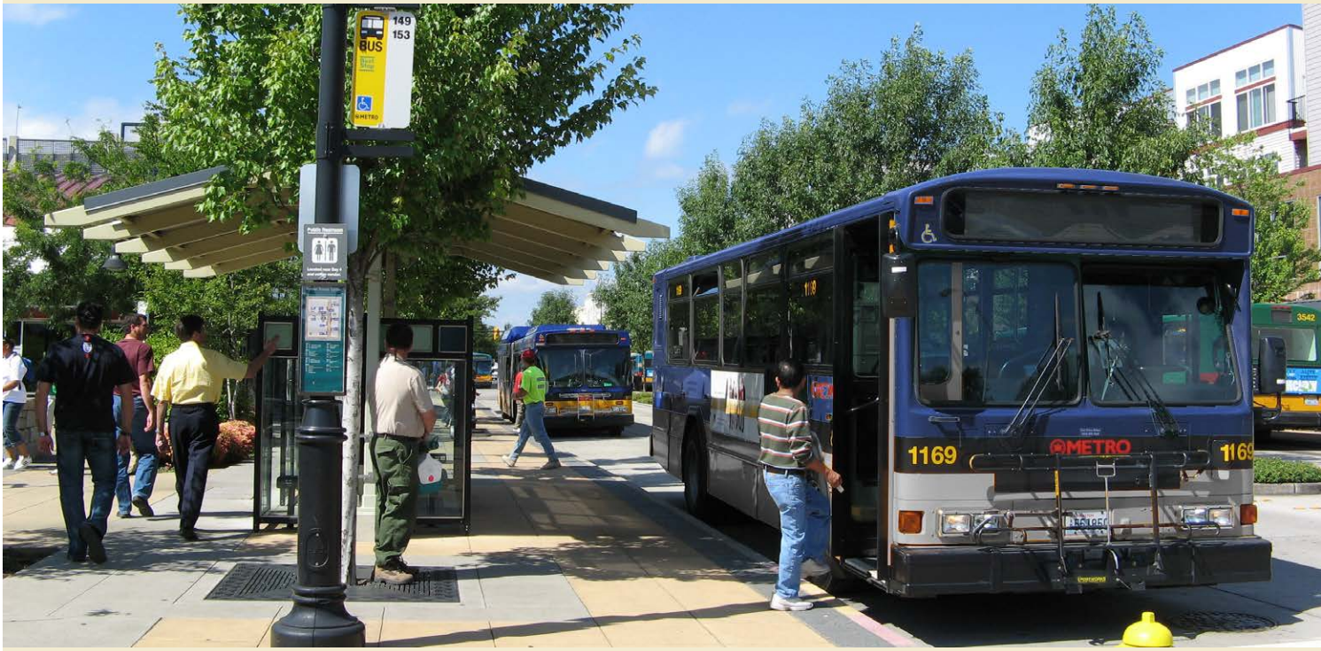
Figure 3.7: Example of an accessible public transit stop with surface texture to identify shelter and stop location
