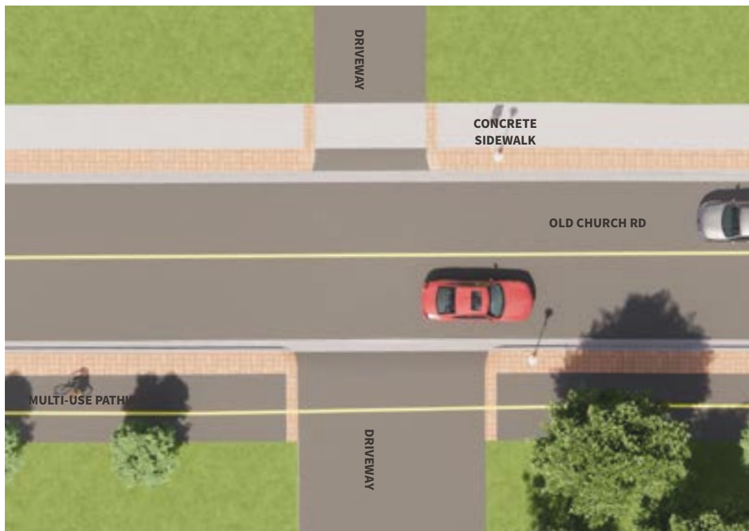
Example of sidewalk and multi-use pathway crossing at driveways
