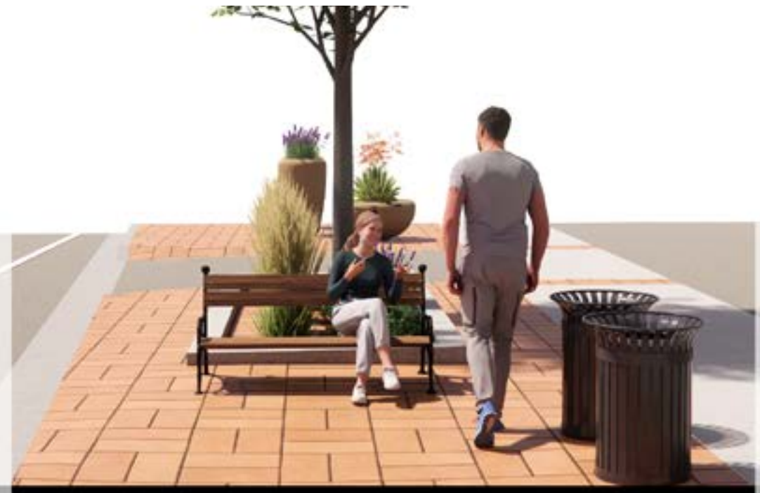
1 METER MIN. IMPRESSED AND COLOURED ASPHALT
