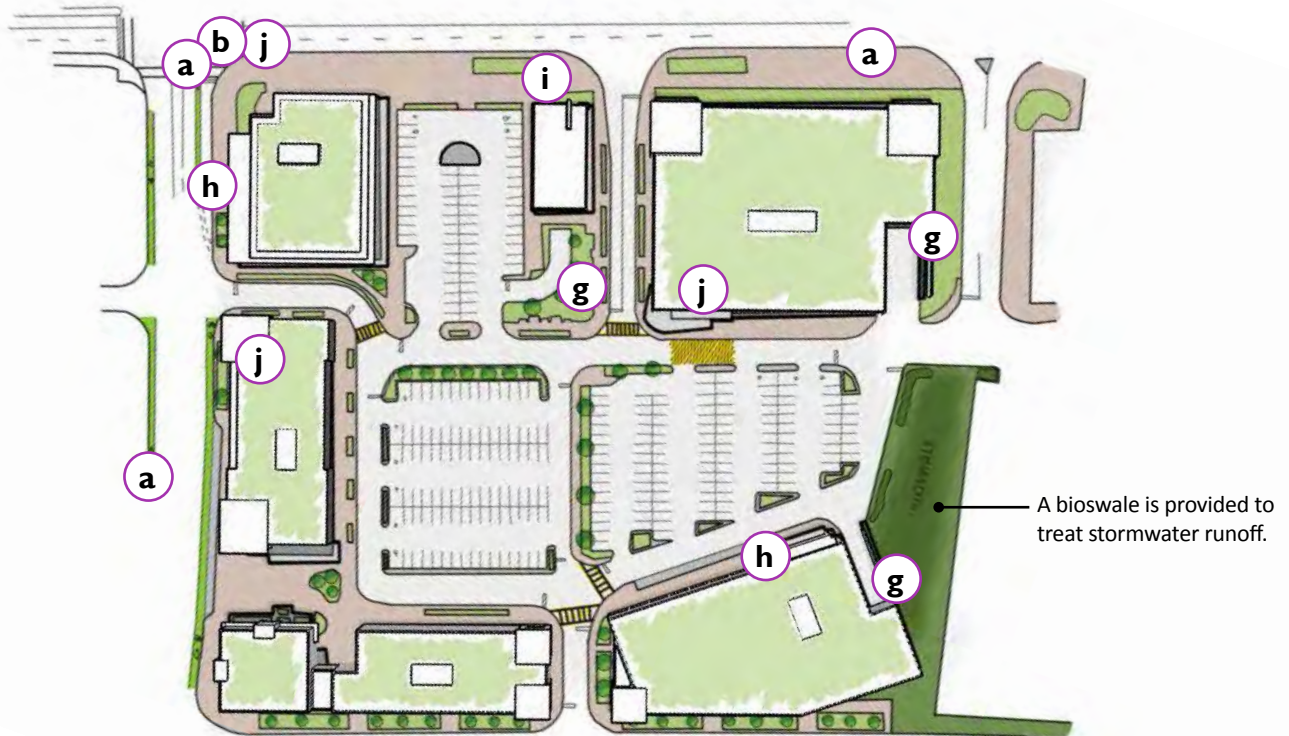
A demonstration plan of a commercial site that addresses the streetscape and integrates green infrastructure in the form of LIDs and green roofs.
