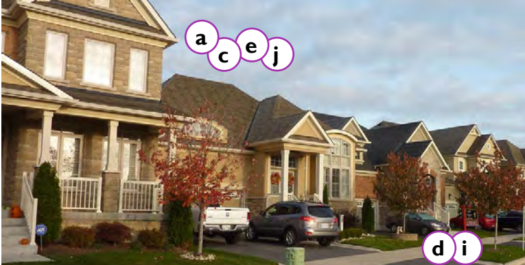
The pairing of garages in Mayfield West maximizes landscaping in front of the dwellings and minimizes the impact on the streetscape.
