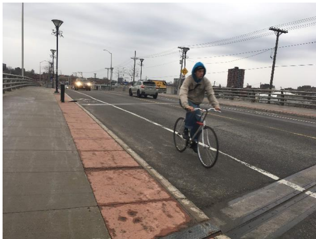
Unbuffered bike lane (Ottawa, ON)
