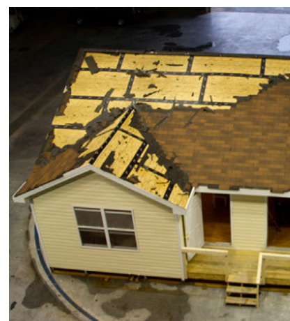
Basic secondary water barrier: Roof deck taping to seal seams between sheathing panels
